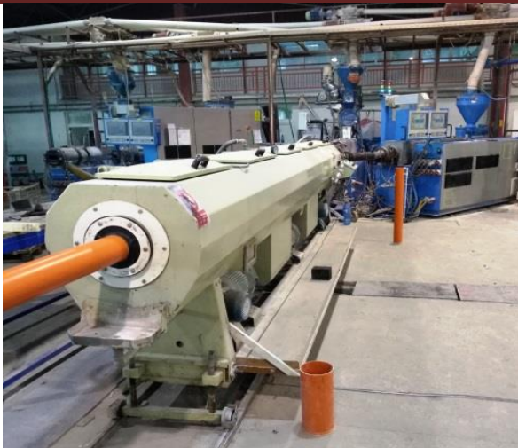
Fig. 3 Extruders for the production of PVC pipe
